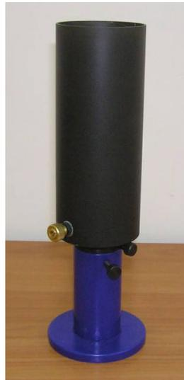
Fig. 8. Cylinder reservoir with illuminators.
