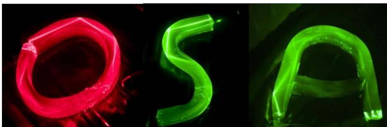
Figure 1: Total internal reflection occurring in gelatine waveguides
