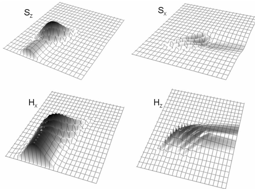
**Fig. 2** Visual representation of the distribution of i) the longitudinal ( $S_z$ ) and transverse ( $S_x$ ) components of the Poynting vector and ii) the magnitude  $H_x$  and the  $H_z$ -fields. The redirection of energy in the X-direction is associated with a transfer of energy from the  $H_x$  to the  $H_z$  component of the magnetic field.
