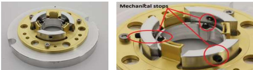
**Fig. 4.** Left, designed and manufactured tool for the lens positioning during soldering process. Right, detail of the spring-type mechanical stops that secured the lens center accuracy.
