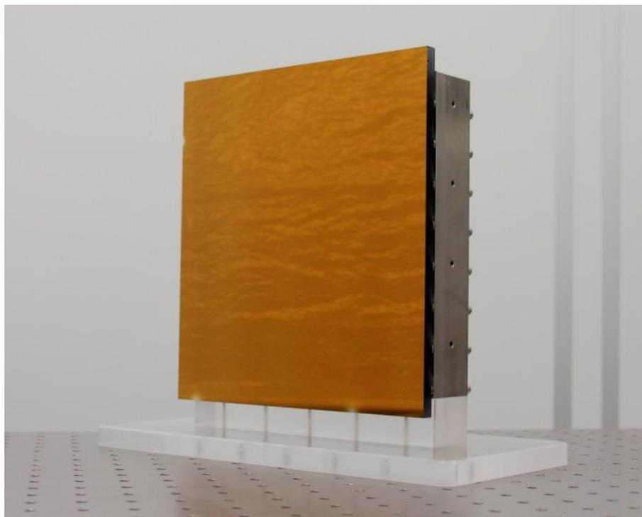
**Fig. 2.** 228x210 mm<sup>2</sup> sample mirror with 80 actuators.
