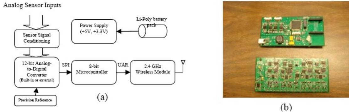
Figure 9. (a) Schematic diagram of the wireless platform developed for the system integration; (b) photograph of the wireless boards developed at UAF.
