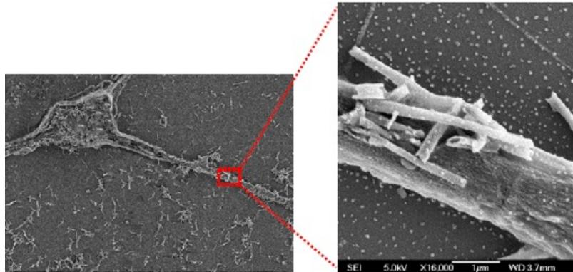
Figure 3. SEM micrographs of magnetic nanotubes attached to the surface of a neurite.
