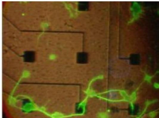
Figure 6. Fluorescent microscope images of neurons cultured on nanowire electrodes
