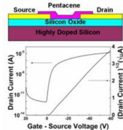
Figure 8. (a) Schematic cross-sectional view of a bottom-contact pentacene TFT without encapsulation. (b) transfer characteristic, measured at RT, of such a bottom-contact pentacene TFT with a channel length and width of 60 and 300  $\mu\text{m}$ , respectively.
