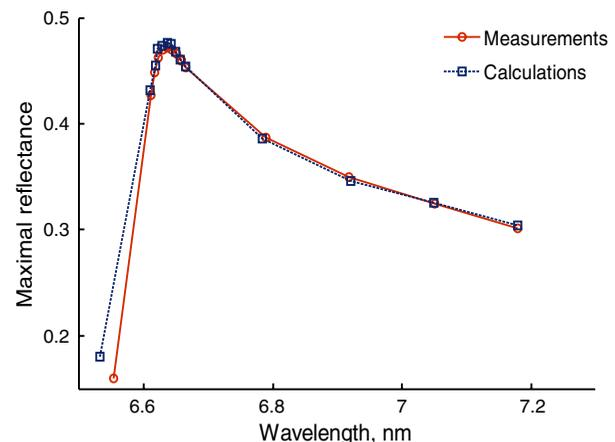
**Fig. 3** Measured and fitted peak reflectivity for a 150 period LaN/B<sub>4</sub>C multilayer mirror. The mirror had a lateral gradient in periodicity. The data points represent the maximum reflectance and corresponding wavelength at various positions on the mirror.
