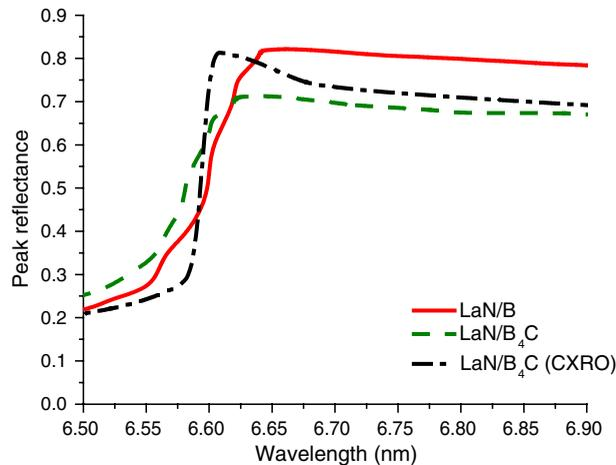
**Fig. 1** Peak reflectivity of a perfect LaN/B multilayer mirror calculated using measured B optical constants (16) (line) and a LaN/B<sub>4</sub>C multilayer mirror calculated using measured (17) (dashed) and Henke (13) (dashed-dotted) optical constants.
