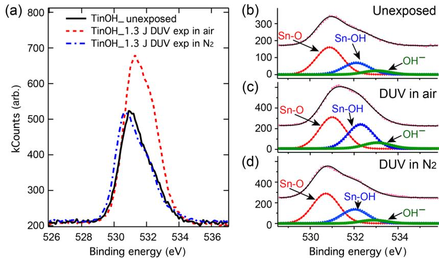
**Fig. 4** The O  $1s$  core-level spectra for TinOH unexposed sample, sample exposed in air, and sample exposed in  $N_2$ . (a) Core-level spectra sharing the same scale on the ordinate axis. (b)–(d) Least squares fits for each sample using the three-component model described in the text.
