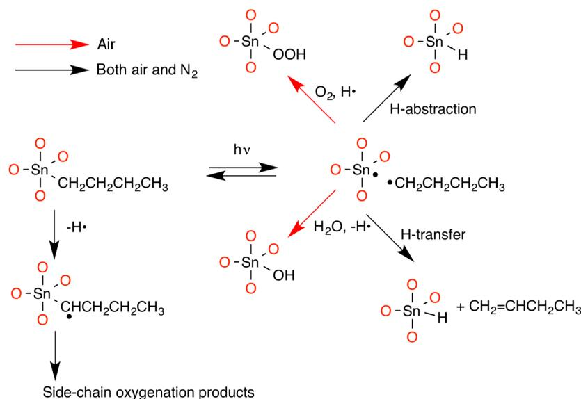
Fig. 6 Proposed photochemical reactions for TinOH exposed to DUV in air and N<sub>2</sub>.
