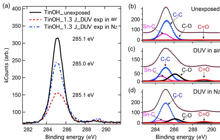
**Fig. 5** (a) C 1s core-level spectra for TinOH unexposed sample, TinOH DUV-exposed in air, and TinOH DUV-exposed in N<sub>2</sub>. (b)–(d) Fits for each sample using the four-component model described in the text.
