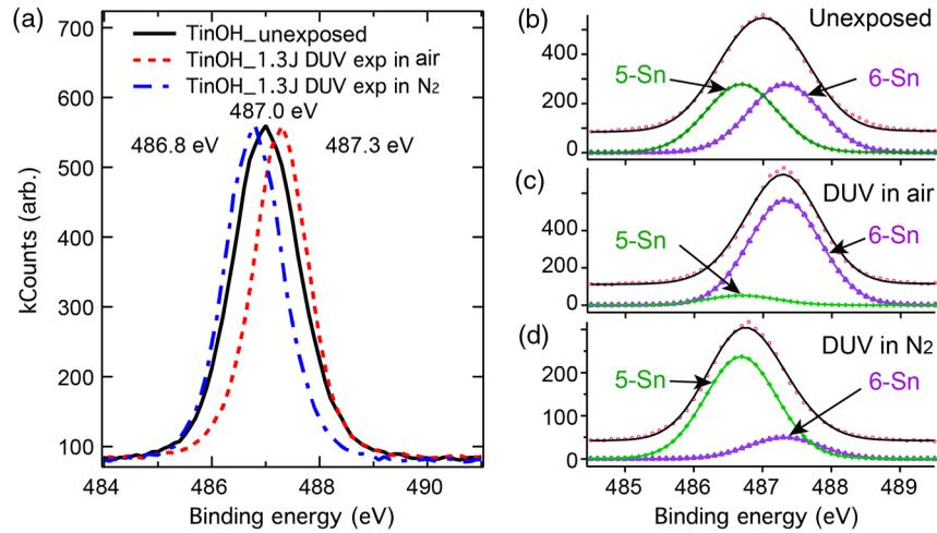
**Fig. 3** Sn  $3d_{5/2}$  core-level spectra for TinOH unexposed sample, TinOH DUV-exposed in air, and TinOH DUV-exposed in  $N_2$ . (a) Core-level spectra sharing the same scale on the ordinate axis. (b)–(d) Fits for each sample using the two-component model described in the text.
