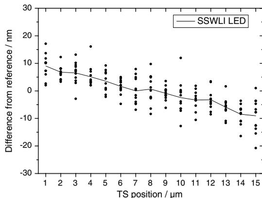
**Fig. 4** Stroboscopic light-emitting diode results—scatter of individual results and their mean (solid line), as differences from the reference values measured with symmetric differential heterodyne laser interferometer.
