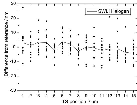
**Fig. 5** Halogen light results—scatter of individual results and their mean (solid line), as differences from the reference values measured with symmetric differential heterodyne laser interferometer.
