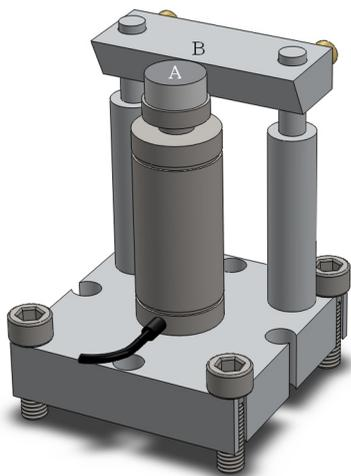
**Fig. 1** Transfer standard (TS). The moving mirror (A) is mounted on a piezo stage. The reference flat (B), its posts, and the baseplate are made of Invar alloy. The height of the TS is 10 cm.
