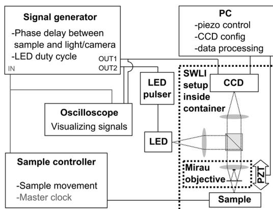
**Fig. 3** Stroboscopic scanning white light interferometer setup. The gray connection from the sample controller is not used in the quasidynamic measurement.
