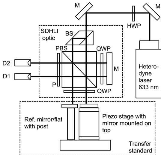
**Fig. 2** TS calibration setup. D1 and D2 are the measurement and reference photodetectors, P is a polarizer, PBS is a polarizing beam-splitter, M is a mirror, QWP is a quarter-wave plate, HWP is a half wave plate, and BS is a beamsplitter.
