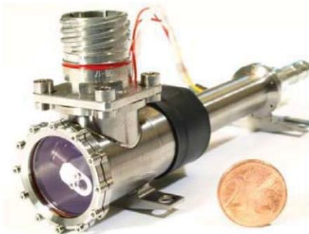
Figure 2. Realization of the laser head prototype.
