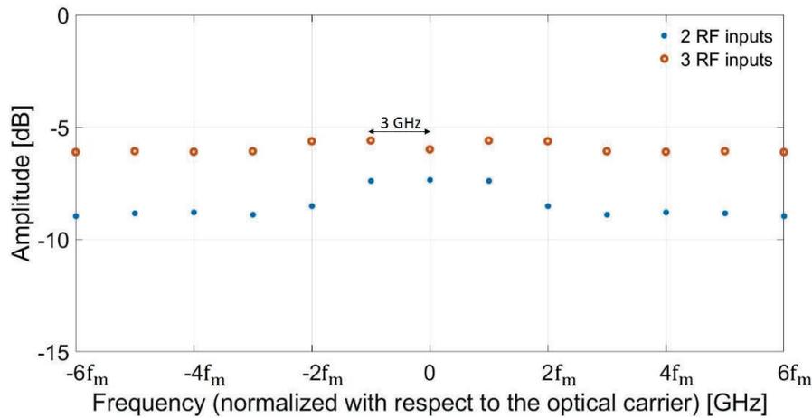
**Fig. 5.** Comparison between the 13 lines output OFC when driving the PM with two or three RF signals. The spacing is set to 3 GHz in both cases and the amplitude difference is 1.6 dB and 0.5 dB, respectively.
