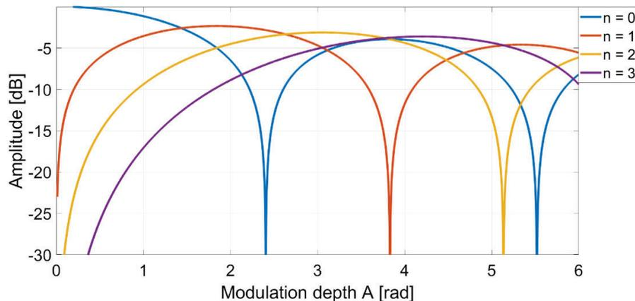
**Fig. 1.** Amplitudes of the first three harmonics in absolute value and logarithmic scale. Because of the Bessel function symmetry, the amplitude of the  $n^{\text{th}}$  harmonic is equal to the amplitude of the  $-n^{\text{th}}$ , where  $n$  is the harmonic order.
