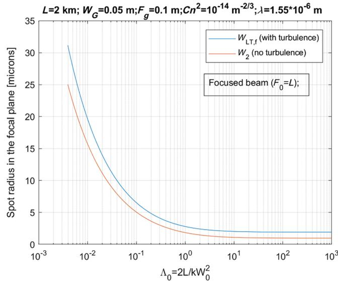
**Fig. 4** Long-term beam spread term  $W_{LT,f}$  (blue) and the diffraction limited spot size  $W_2$  (red) as a function of the diffraction parameter  $\Lambda_0$  for a beam focused on the receiver (Kolmogorov turbulence case). Distance is fixed to the value  $L = 2$  km.
