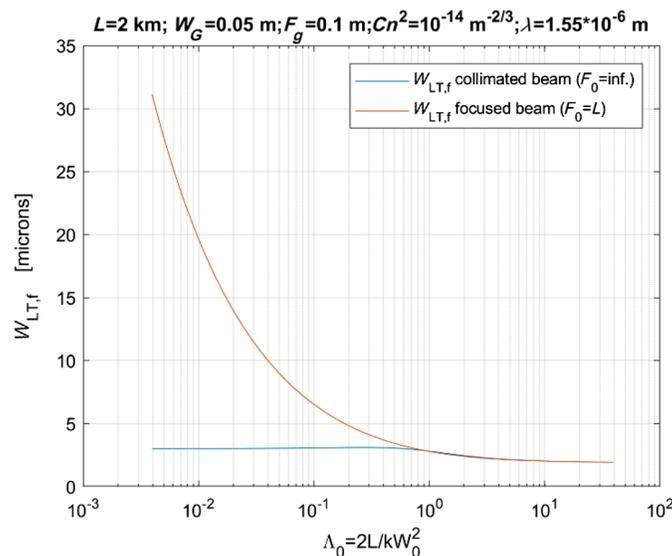
**Fig. 5** Long-term beam spread term  $W_{LT,f}$  as a function of the diffraction parameter  $\Lambda_0$  for both beam geometries: collimated and focused (Kolmogorov turbulence case). Distance is fixed to the value  $L = 2$  km.
