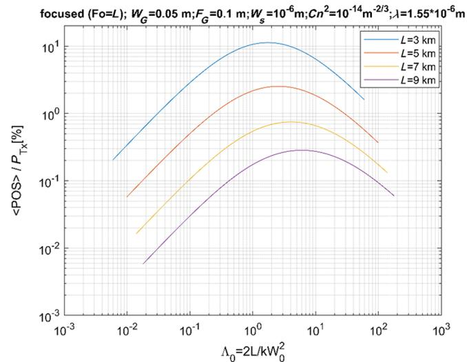
**Fig. 10** Percentage of POS scaled by the transmitted power as a function of the diffraction parameter  $\Lambda_0$  for several distances of the receiver for a beam focused on the receiver (Kolmogorov turbulence case only).
