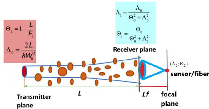
Fig. 1 Free space optical communication scheme.
