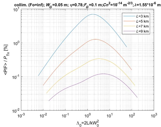
**Fig. 11** Percentage of PIF scaled by the transmitted power as a function of the diffraction parameter  $\Lambda_0$  for several distances of the receiver for a collimated beam at the transmitter (Kolmogorov turbulence case only).
