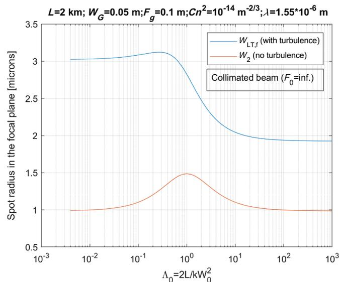
**Fig. 3** Long-term beam spread term  $W_{\text{LT},f}$  (blue) and the diffraction limited spot radius  $W_2$  (red) as a function of the diffraction parameter  $\Lambda_0$  for a beam collimated at the transmitter (Kolmogorov turbulence case only). Distance is fixed to the value  $L = 2$  km.
