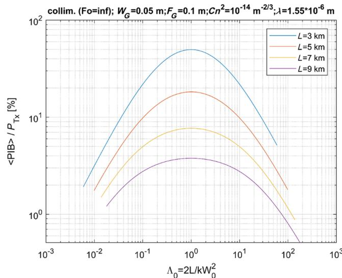
**Fig. 7** Percentage of PIB scaled by the transmitted power as a function of the diffraction parameter  $\Lambda_0$  for several distances of the receiver for a collimated beam at the transmitter (Kolmogorov turbulence case only).
