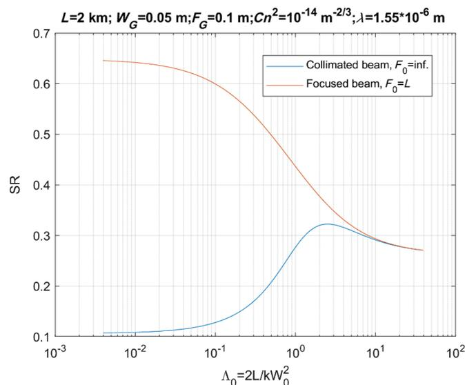
**Fig. 6** SR as a function of the diffraction parameter  $\Lambda_0$  for a beam collimated at the transmitter (blue) or focused on the receiver (red) (Kolmogorov turbulence case only). Distance is fixed to the value  $L = 2$  km.
