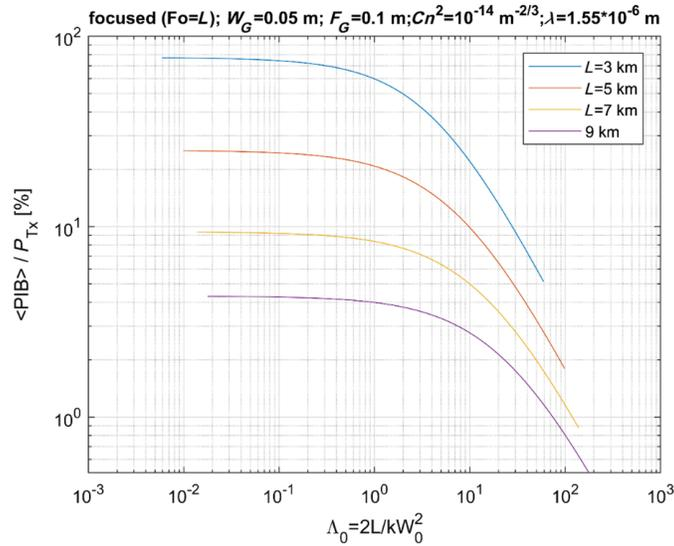
**Fig. 8** Percentage of PIB scaled by the transmitted power as a function of the diffraction parameter  $\Lambda_0$  for several distances of the receiver for a beam focused on the receiver (Kolmogorov turbulence case only).
