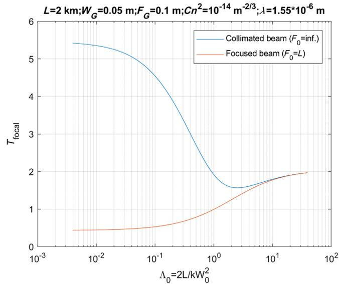
**Fig. 2** Spread term  $T_{\text{focal}}$  as a function of the diffraction parameter  $\Lambda_0$  for a beam collimated at the transmitter (blue) or focused on the receiver (red) (Kolmogorov turbulence case). Distance is fixed to the value  $L = 2$  km.
