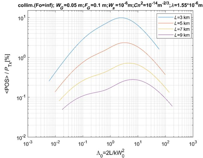
**Fig. 9** Percentage of POS scaled by the transmitted power as a function of the diffraction parameter  $\Lambda_0$  for several distances of the receiver for a collimated beam at the transmitter (Kolmogorov turbulence case only).
