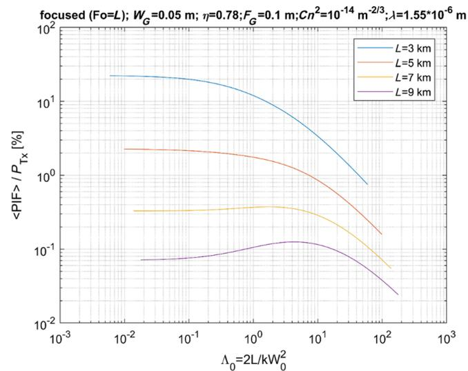
**Fig. 12** Percentage of PIF scaled by the transmitted power as a function of the diffraction parameter  $\Lambda_0$  for several distances of the receiver for a beam focused on the receiver (Kolmogorov turbulence case only).
