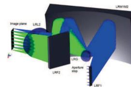
Figure 11: Optical layout of the FM FLEX Low Resolution Spectrometer.
