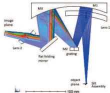
Figure 1: BB layout of the FLEX LRSP.
