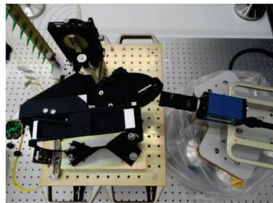
Figure 5: SHS measurement set-up (LRSP in the center, SHS on the right, FISLI at the top)
