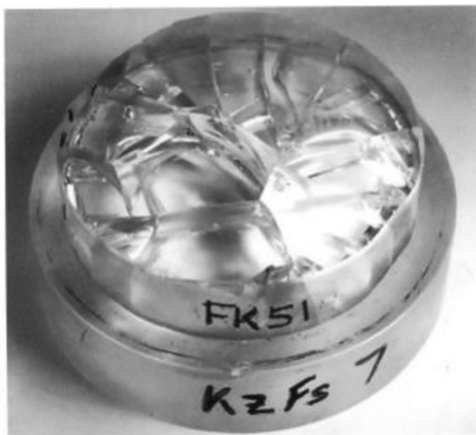
Photograph of a bonded doublet fractured by thermal stress [P. R. Yoder, Jr. and D. Vukobratovich, “Shear stresses in cemented and bonded optics due to temperature changes,” Proc. SPIE 9573, 95730J (2015)].
