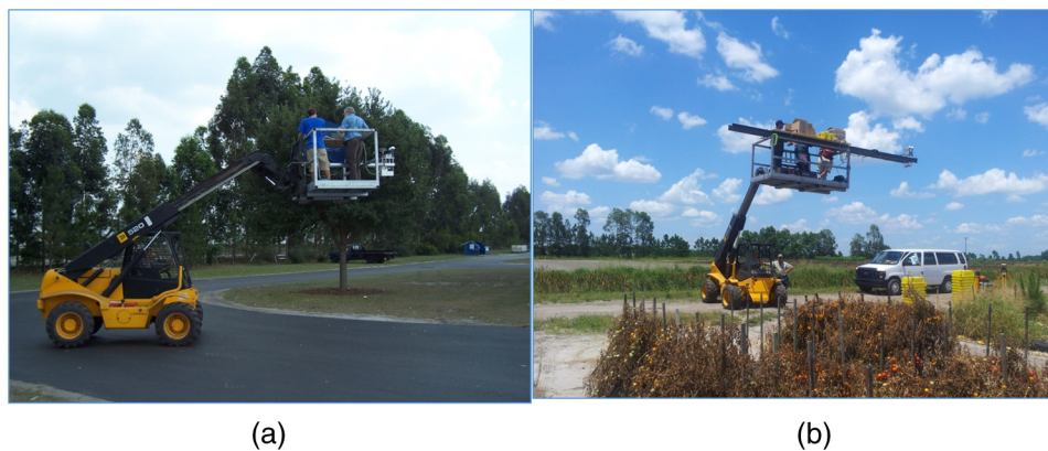
Fig. 3 The MGIS mounted on elevated platform (forklift tractor). Images collected over: (a) pavement road surface and (b) agricultural beds.
