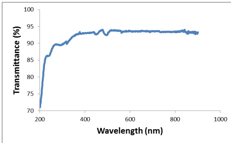
Figure 4. Measured transmittance of a layer of CeO<sub>2</sub> film on quartz fabricated with 25 nm nanoparticles.
