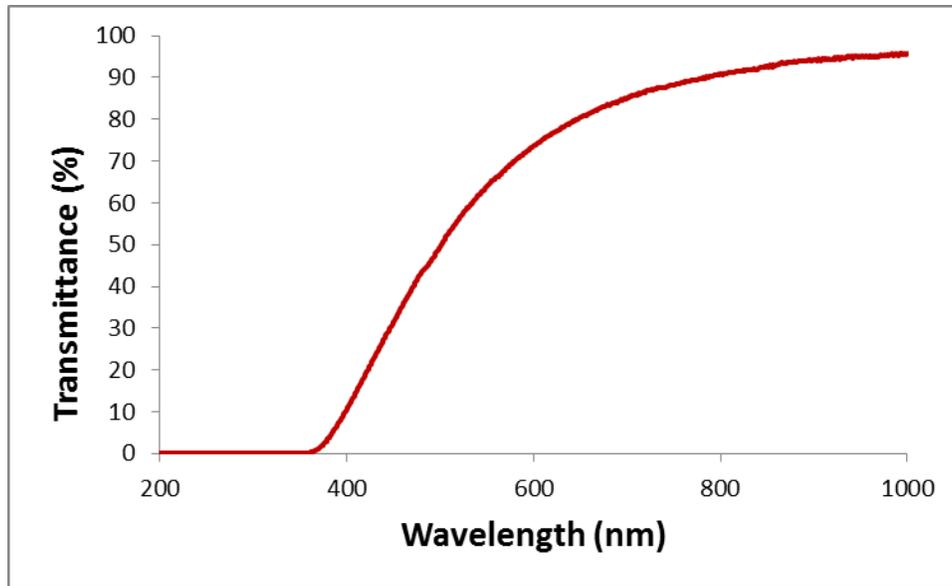
Figure 3. Measured transmittance of cerium oxide aqueous solution.
