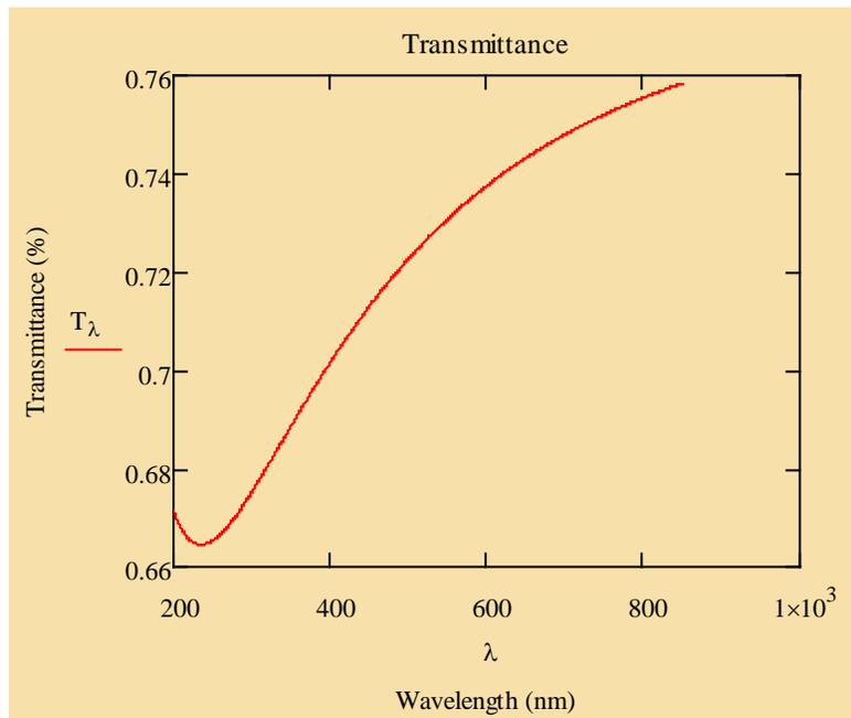
Figure 1. Calculated transmittance for a 25 nm layer of CeO<sub>2</sub> on quartz substrate.
