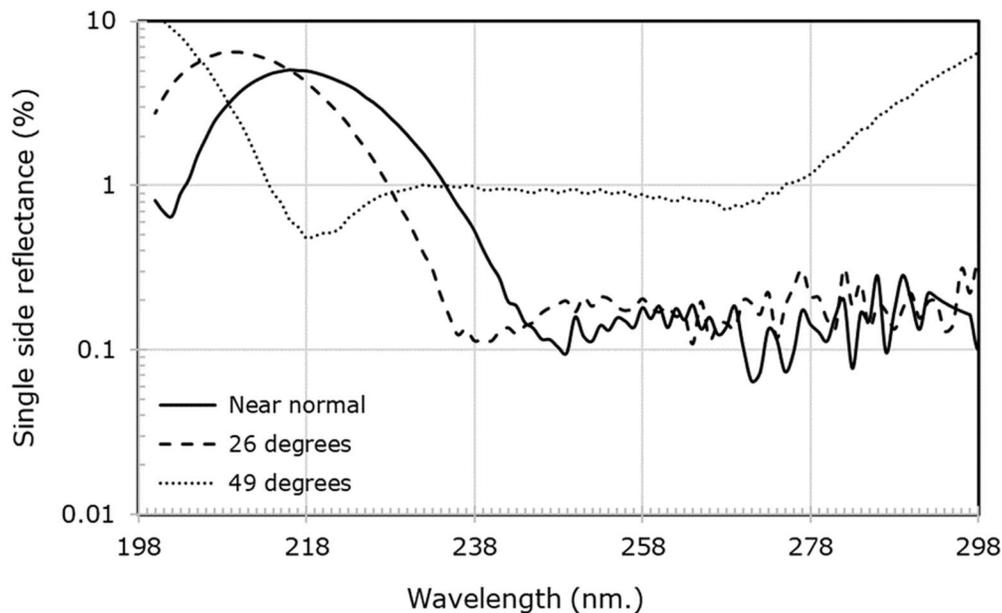
Fig. 1. Spectral performance of a multilayer  $\text{Al}_2\text{O}_3/\text{MgF}_2$  AR coating optimized for a wide angle of incidence.
