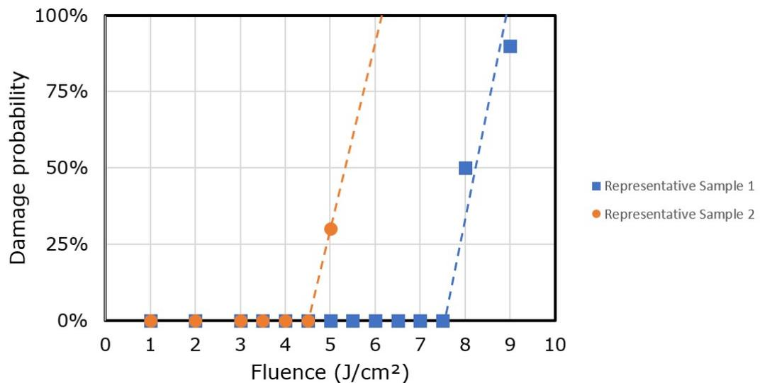
Fig. 3. LDT results for multilayered Al<sub>2</sub>O<sub>3</sub>/ MgF<sub>2</sub> coatings at 248 nm.
