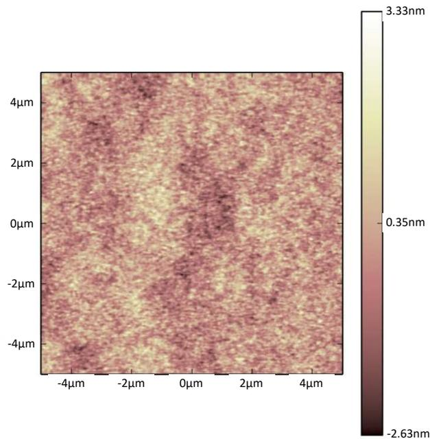
Fig. 2. AFM image of multilayered Al<sub>2</sub>O<sub>3</sub>/MgF<sub>2</sub> antireflection coating on a commercially polished substrate.
