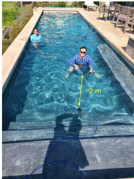
Figure 2. Picture of the pool test site. The 30 MHz SEW signal is transmitted using an underwater surface wave antenna using 20 mW (13dBm) transmit power. The measured water salinity in the pool was 0.2%, which corresponds to 20 cm skin depth at 30 MHz.
