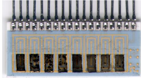
Figure 1. A sensor substrate used in the JPL ENose. Eight polymer-carbon black composite sensors are drop cast onto a masked substrate. Four substrates are used in a complete array.
