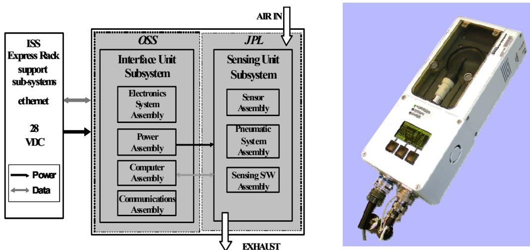
Figure 5. The Third Generation ENose. The block diagram on the left shown the different subsystems and the interfaces to ISS. The device shown on left was autonomous. It has a volume of 3.6 L, a mass of 3.4 kg and used 8 watts average power and 15 watts peak power. Power was provided by ISS; all other functions are integral to the device.
