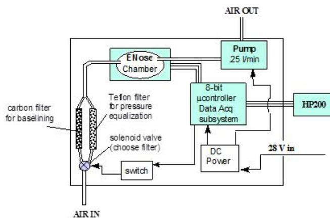
Figure 2. A block diagram of the arrangement of the First Generation JPL ENose. Subsequent version of the JPL ENose had the same basic components and set-up.
