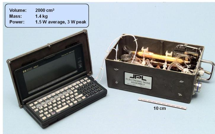
Figure 3. The First Generation JPL ENose flight unit. The palm top computer fit inside the container and was used for device control and data acquisition. This device had a volume of 2.0 liters, a mass of 1.4 kg and used 1.5 watts average power, 3 watts peak power.
