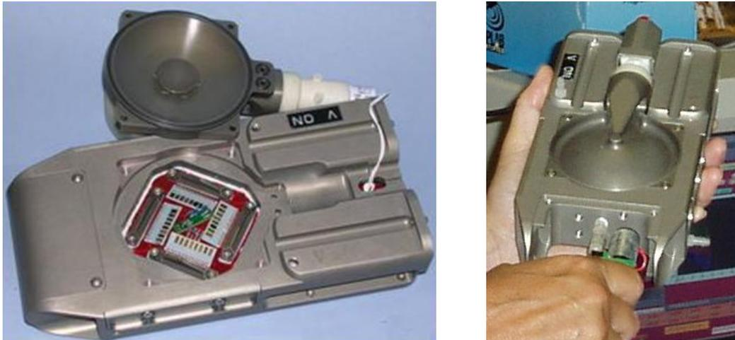
Figure 4. The Second Generation ENose. The ENose is operated by an outboard computer. Power may be provided by a battery pack or line current. This device has a volume of 750 cm<sup>3</sup>, a mass of 800 g and used 1.5 watts average power, 3 watts peak power.
