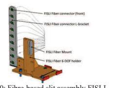
Figure 10: Fibre-based slit assembly FISLI.
