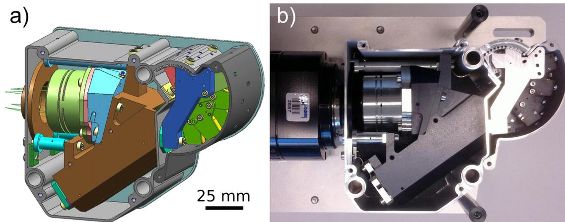
**Fig. 1.** a) Mechanical design drawing of the opto-mechanical unit of SPEX. The nine viewports are the green units on the right, the grating is mounted in the cyan compartment and the imaging lenses are embedded in the light green housing. The focal plane lies just outside the structure. b) Picture of the realization of SPEX showing the black anodised viewports on the right and the detector mounted to the structure on the left.
