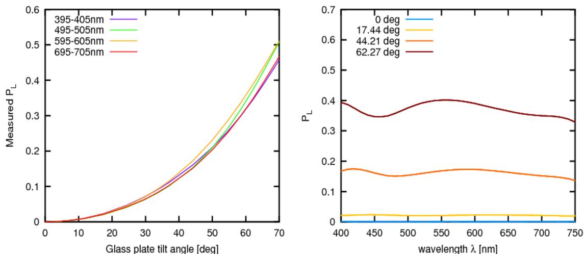
**Fig. 3.** a) Measured  $P_L$  of the stimulus plotted as a function of glass plate tilt angle for four different wavelengths. b) Spectral variation of  $P_L$  plotted for four different glass plate tilt angle.
