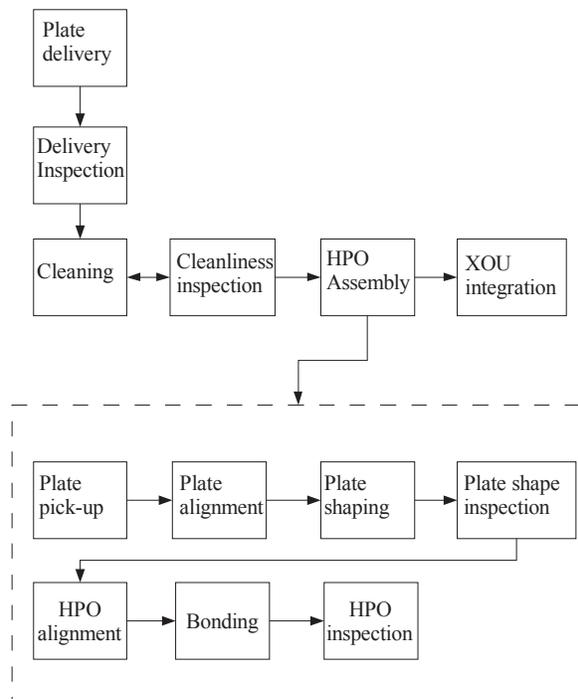
Fig. 6. The workflow of the production process starting from plate delivery up to its integration into an XOU.
