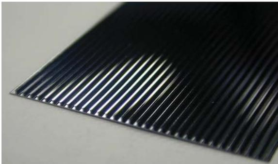
Fig. 1. A structured Si wafer that forms a ribbed mirror plate and the base material for the X-ray optics.
