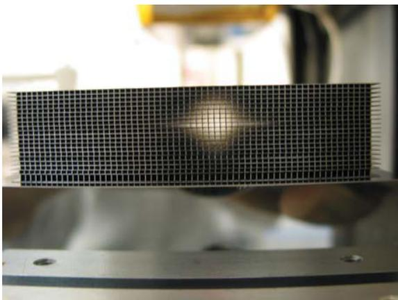
Fig. 4. Photograph of a High Performance Pore Optics on top of a polished former as recently produced by cosine Research.
