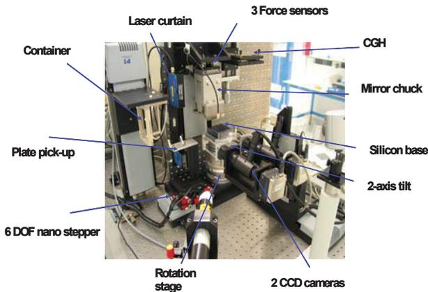
Fig. 3. The X-ray Optics Assembly Tool (XOAT) as installed in the cleanroom of the Cosine Research Centre in Leiden.
