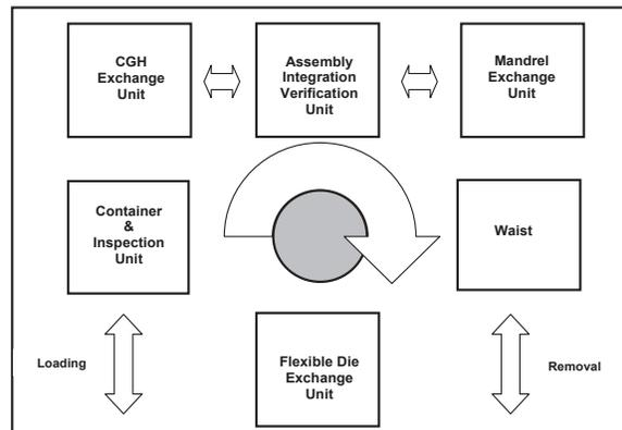
Fig. 9. Conceptual layout of the assembly robot. The core element in the centre is used to extract, move and supply all mirrors to the assembly and integration unit.
