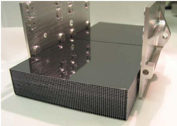
Fig. 7. Integration jig to assemble a pair of HPOs into an XOU. The two HPOs are co-aligned and integrated using brackets to form a Wolter-I X-ray lens.
