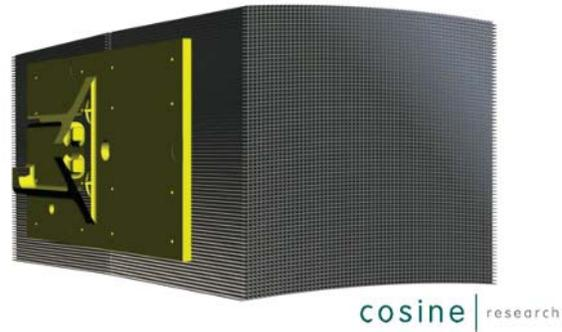
Fig. 5. Layout of a larger X-ray Optical Unit that is made of two High Performance Pore Optics.
