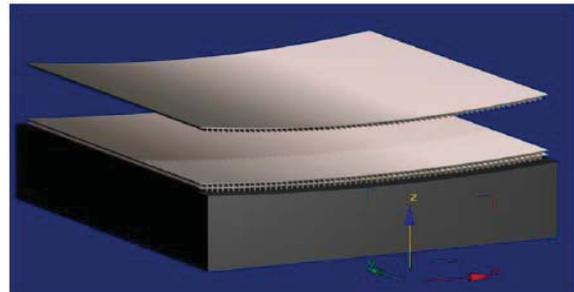
Fig. 2. Visualisation of the assembly concept. Structured Si plates are bent into a highly accurate cylindrical shape and are stacked successively on top of each other.
