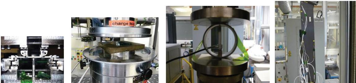
Figure 2. LEFM – Thales Alenia Space’s mechanical test lab can perform a wide variety of tests: 4-point bending, ring-on-ring, O- and C-ring, tensile
