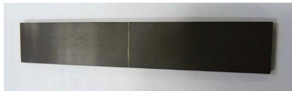
Figure 8. Silicon nitride sample with a brazed junction at the middle of the sample, for 4-point bending tests
