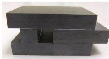
Figure 9 Silicon nitride sample with brazed junctions for double shearing tests
