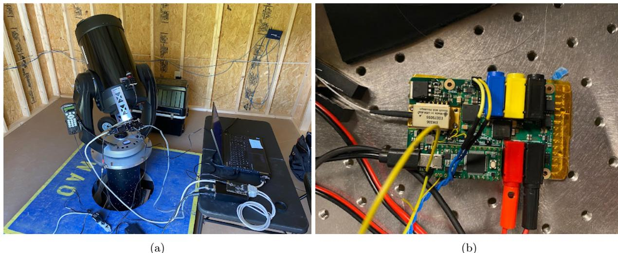
Figure 2: a) PorTeL optical ground station located within its observatory shed at MIT Wallace Astrophysical Observatory. Image credit: Peter Grenfell b) Beacon driver board for CLICK mission. Image credit: Nick Belsten
