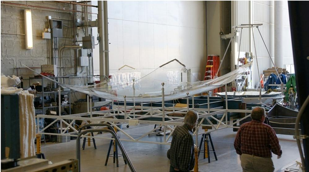
Figure 7. Shaped, uncoated dish 3.1 m square made at the University of Arizona Mirror Lab.
