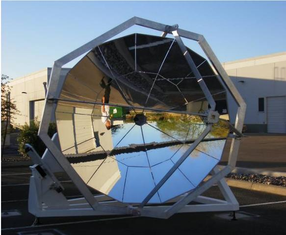
Figure 5. 2.5 m in diameter solar reflector prototype, with segments shaped from 4 mm thick float glass.
