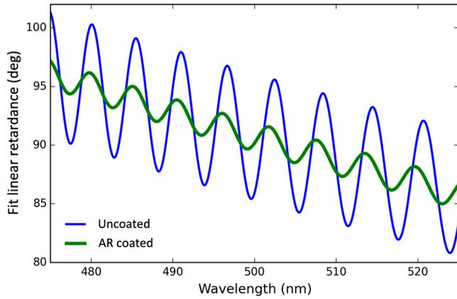
**Fig. 6** The linear retardance fit to a zero-order quartz crystal retarder of  $13.587 \mu\text{m}$  physical thickness. Blue shows uncoated. Green shows antireflection coated. The blue curve can be compared with Clarke.<sup>49</sup> We use the Sueoka<sup>10</sup> revised birefringence measurements, and we get a slightly different retardance than when using the CVI refractive indices giving  $13.587 \mu\text{m}$  as the exact zero-order retardance thickness for 500-nm wavelength.
