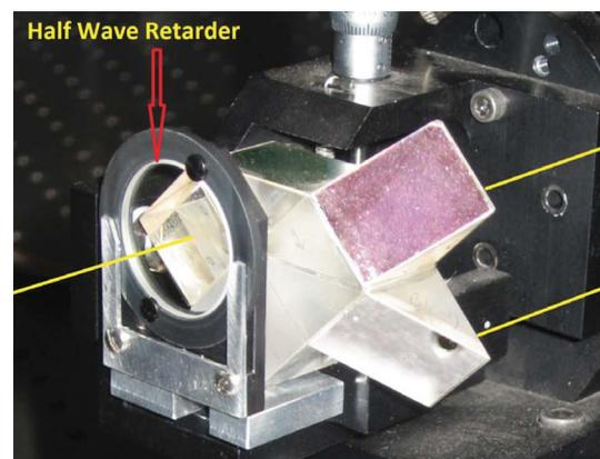
**Fig. 10** The half-wave retarder mounted with the SPINOR polarizing beam splitter near the slit. Courtesy Doug Gilliam, DST staff.
