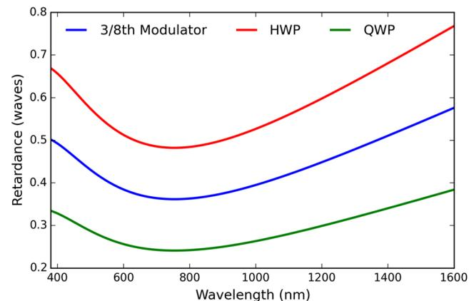
**Fig. 9** The linear retardance predicted for the three SPINOR bicrystalline achromats. SPINOR retarder designs at 633 nm wavelength are to 1/4-wave, 3/8-wave, and 1/2-wave retardance. The 1/4 wave is shown in green with crystals at (0.960209 and 1.098837 mm) thickness. The 3/8-wave retarder is shown in blue with crystals of (1.438883 and 1.648256 mm) thickness. The 1/2-wave retarder is shown in red with crystals at (1.920417 and 2.197675 mm) thickness.
