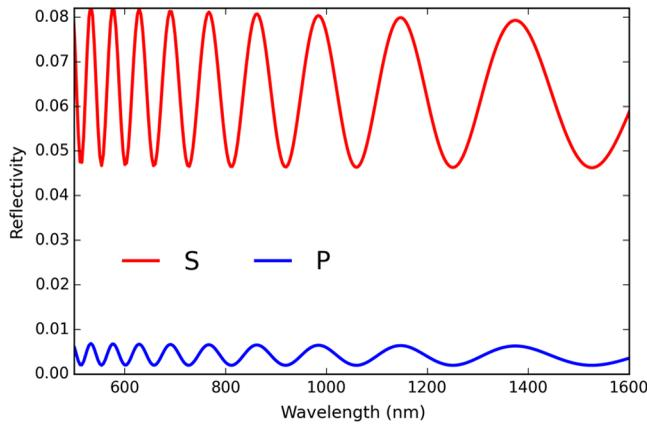
**Fig. 2** The reflectivity for the thick isotropic  $\text{MgF}_2$  coating on a fused silica window at a 45-deg incidence angle. The reflectivity curves oscillate about their average values of 6.43% for  $S$ - and 0.43% for  $P$ -.
