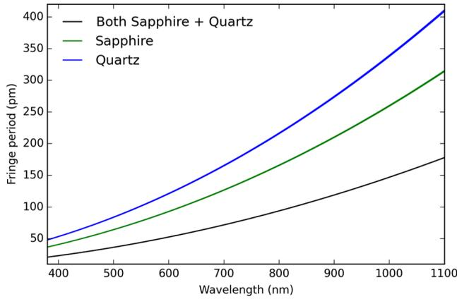
**Fig. 11** The fringe period predicted using the optical thickness of the quarter-wave retarder and Eq. (4) for period ( $\lambda^2/2dn$ ). The o- and e-beam fringe periods are both plotted, but are within the thickness of the plotted line. Blue shows the fringe through the quartz crystal, green shows the sapphire crystal, and black shows both crystals together as a bicrystalline achromat. See text for details.
