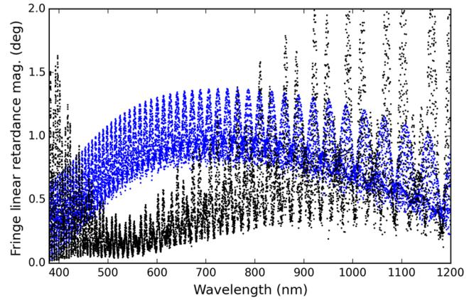
**Fig. 12** The amplitude of the linear retardance fringes in narrow spectral bandpasses of  $R = 10,000$  spectral sampling for the SPINOR 3/8-wave modulator. Black is the linear retardance fringe magnitude using a  $20\text{-}\mu\text{m}$  air gap and a single-layer antireflection coating. Blue shows an uncoated model with crystals optically contacted. See text for details.
