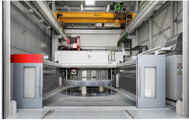
**Fig. 18** Schott Glass 5-m, 5-axis CNC machine center-loaded with a 4.5-m glassy ZERODUR<sup>®</sup> blank.
