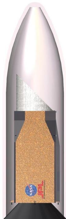
**Fig. 12** Payload fits in SLS 8.4 m fairing.
