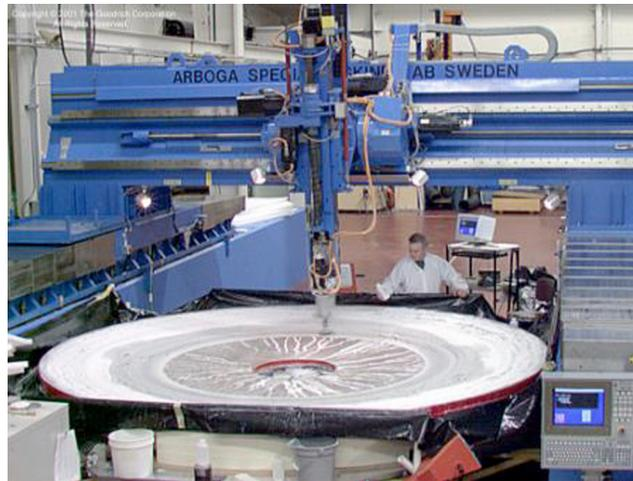
**Fig. 19** Collins Aerospace computer-controlled manufacture of 4.2-m SOAR PM.
