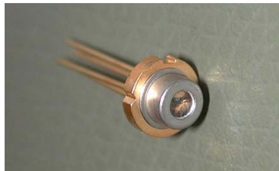
Fig. 1. SLED packaged into a TO-56 housing.
