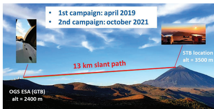
Figure 1. Summary of the FEDELIO experiment (© G. Artaud). The ground station emulator (GTB) is inside the ESA OGS, while the satellite emulator (STB) is in Teide cable car station.
