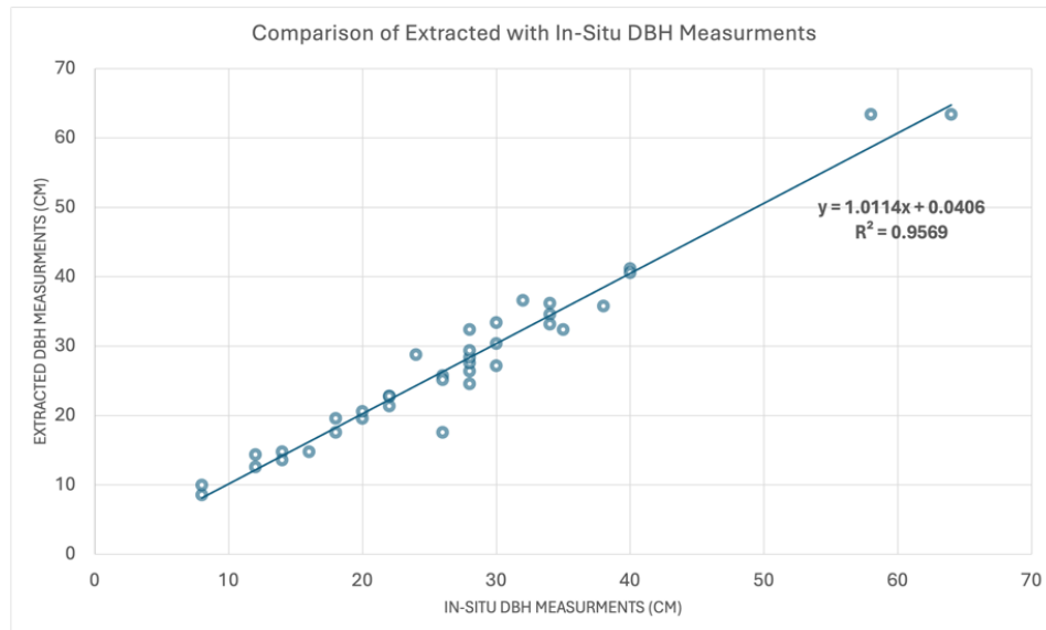
Figure 17. Comparison of the DBH index for plot 3 in the Strofilia forest (ID3). The chart shows a strong correlation ( R^2 \approx 0.957 ) between in situ DBH measurements and those extracted automatically by the 3D Forest application, indicating high accuracy of the automated method.
