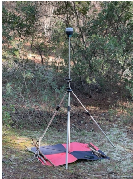
Figure 7. Emlid Reach RS2 GNSS Receiver. The receiver is positioned on a GCP, recording RAW data.
