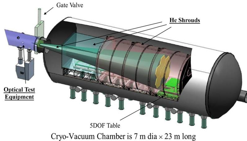
**Fig. 24** Webb mirror testing in MSFC's X-ray and cryogenic facility (XRCF).
