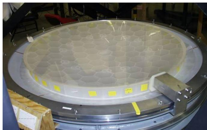
**Fig. 28** Kepler primary mirror on air bladder.
