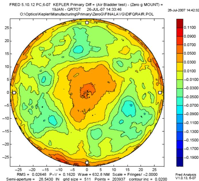
**Fig. 29** Difference between air bladder test and 108 point zero-g mounts is 16.4 nm rms.
