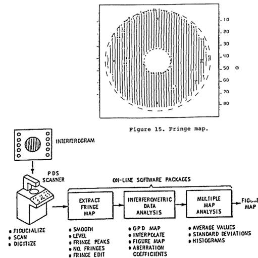
Figure 14. Interferogram analysis facility.
