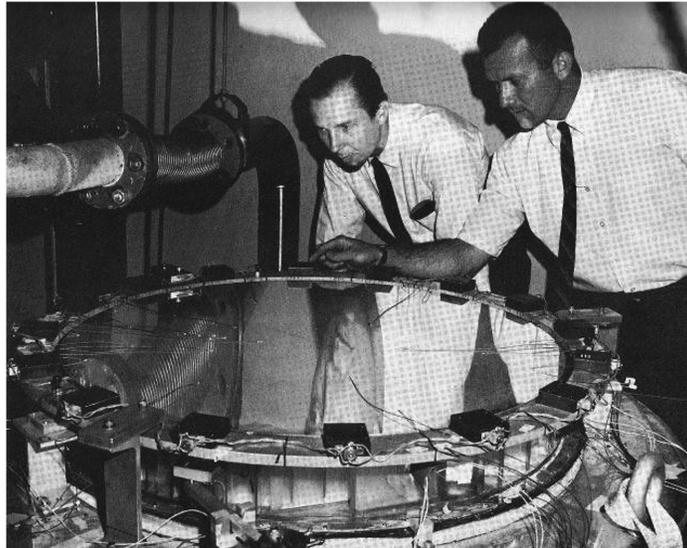
**Fig. 15** OAO-C Princeton mirror in thermal/deformation test.
