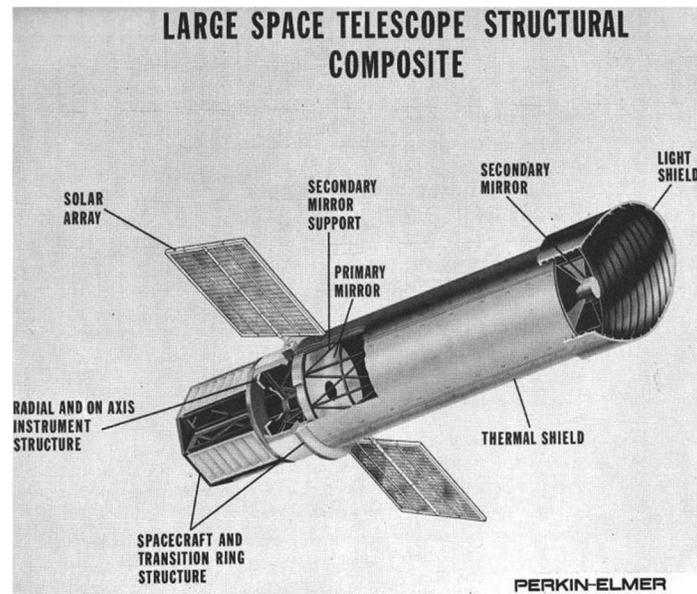
Fig. 6 Free-flying 3 m telescope.<sup>14</sup>
