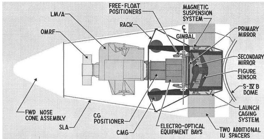
Fig. 4 Stowed launch configuration for Saturn 1B.<sup>12</sup>
