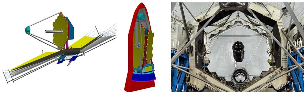
**Fig. 9** TRW/BATC drop leaf table concept used hex segments similar to the Keck Telescope.
