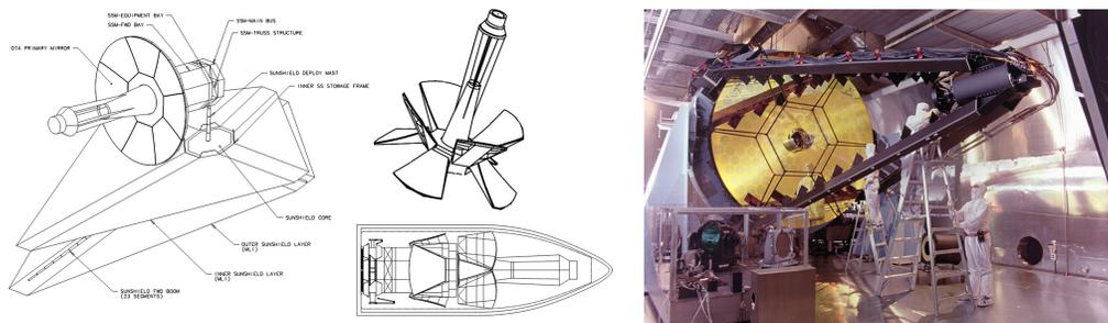
**Fig. 10** LMCO/Raytheon fold-forward/fold-Aft concept was similar to the Air Force LAMP telescope.
