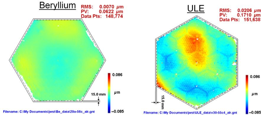
**Fig. 18** Cryo-stability Be versus ULE.
