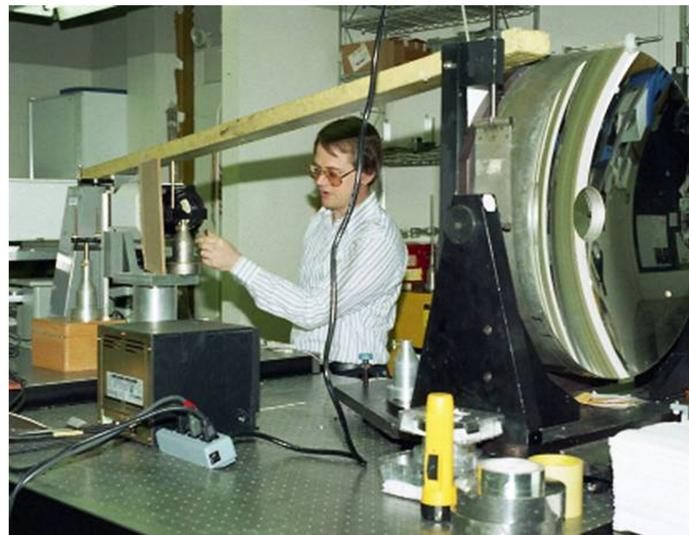
**Fig. 23** Testing spitzer secondary mirror (courtesy Goodrich).
