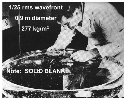
**Fig. 12** Stratoscope II mirror.
