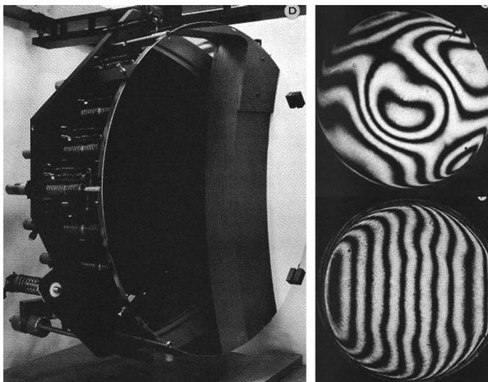
**Fig. 17** 76 cm thin facesheet deformable mirror.
