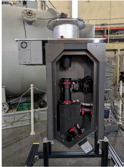
Fig. 10 ETSI during assembly at McDonald Observatory. The red split rings holding the lens barrels are visible. The multi-choic and prisms are mounted inside the black 3D-printed cover with the Texas A&M Logo. The black extruded aluminum frame holding ETSI can be rolled around the observing floor and is removed once ETSI is mounted. Spring-loaded casters allow for any misalignment as ETSI is lifted to the back of the telescope for mounting.
