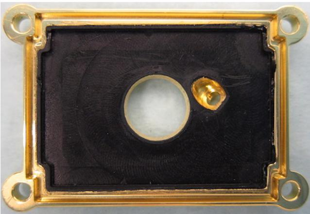
**Fig. 13** The inside surface of a CTS lid with a 1-mm-thick layer of Stycast® 2850 loaded with lampblack carbon powder.
