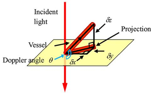
Fig. 2 Defined vessel Doppler angle.
