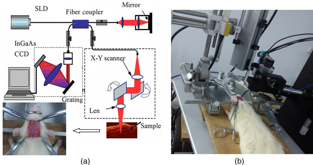
**Fig. 1** (a) Schematic of our OCT system used to obtain hemodynamic MCA parameters. SLD: superluminescent diode, CCD: the charge coupled device. (b) Microinjection device for injecting ET-1.
