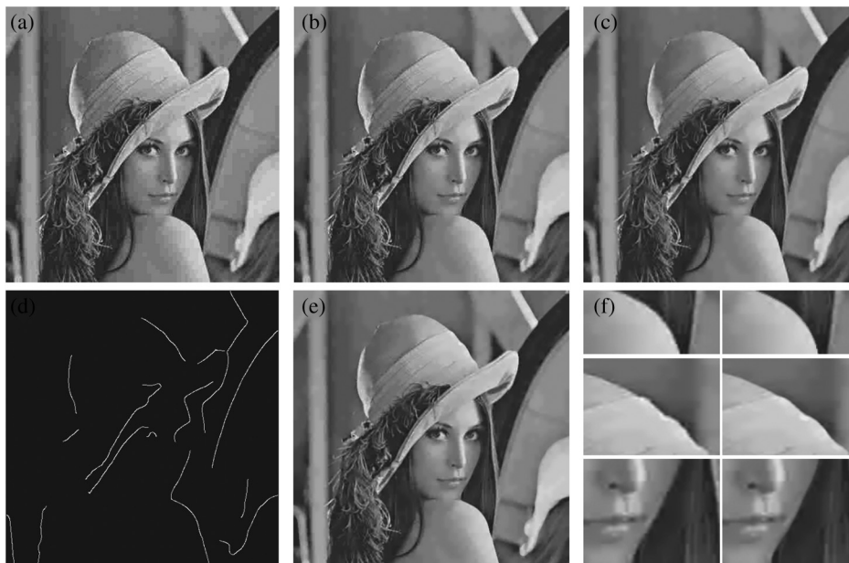
Fig. 5 Deblocking and edge regeneration results. (a) Input image PSNR = 30.40. (b) Result of guided filter without reducing discontinuities between the neighboring blocks. (c) Result after deblocking algorithm [applying Eqs. (1)–(4) and guided filter]. (d) Edge map of Lena by using Canny edge detection on (c). (e) Image after proposed edge regeneration, PSNR = 30.56 dB. (f) Shoulder, hat, and cheek of Lena before (left side) and after (right side) applying proposed algorithm.
