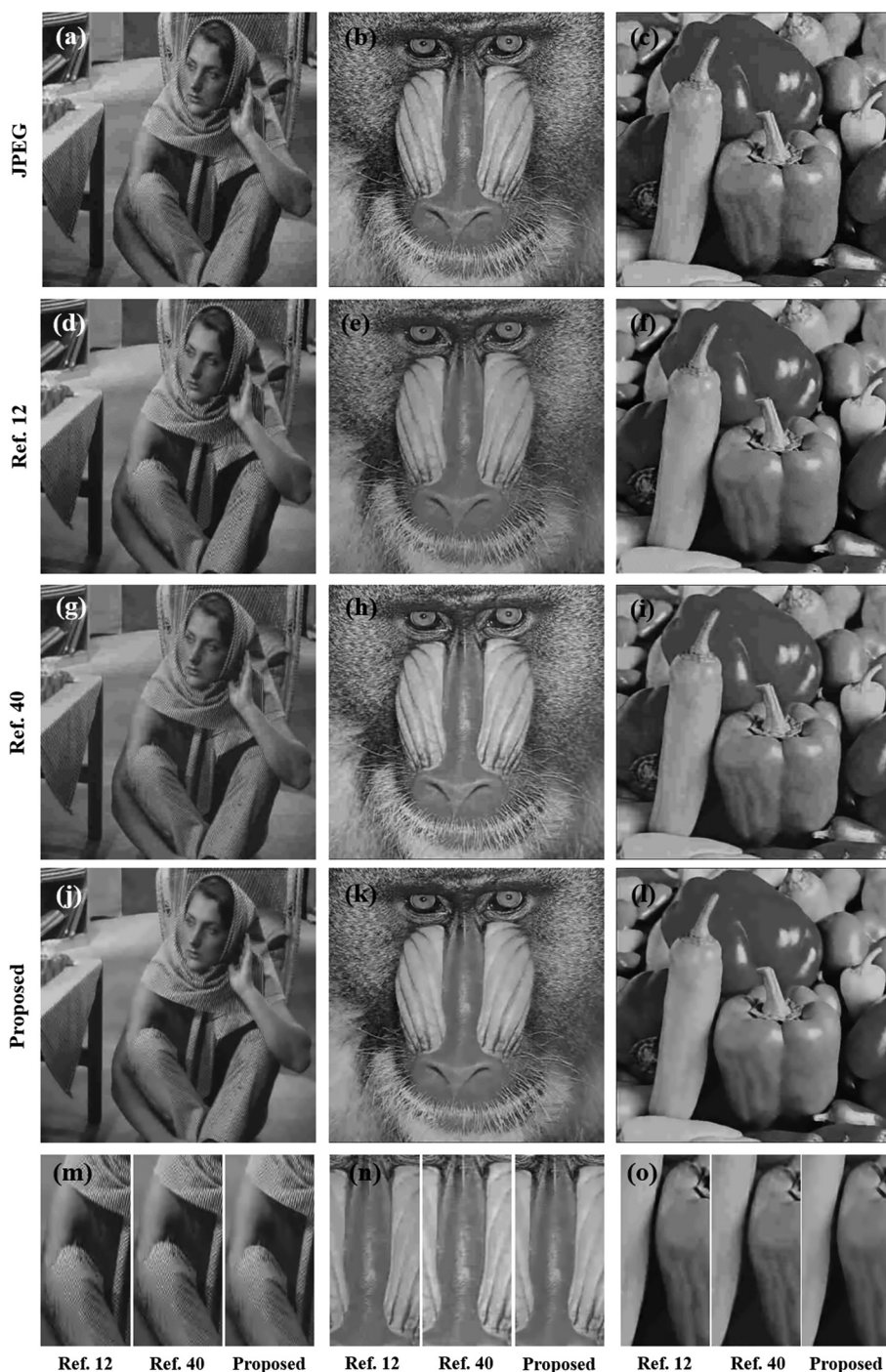
Fig. 10 Subjective quality comparison of the images Barbara , baboon , and peppers compressed at quality factor Q = 10 . (a), (b), and (c) JPEG compressed images, PSNR = 26.33, 23.43, and 30.72 dB. (d), (e), and (f) the result of Ref. 12, PSNR = 26.02, 23.53, and 30.91 dB. (g), (h), and (i) the result of Ref. 40, PSNR = 26.03, 23.67, and 30.90 dB. (j), (k), and (l) the results of our proposed algorithm, PSNR = 26.44, 23.68, and 31.28 dB. (m), (n), and (o) the two left images are close-up of the results from Refs. 40, 12 and right image is a close-up of the result from our proposed algorithm.
