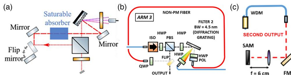
**Fig. 11** Schematic of the starting arms: (a) the starting arm containing a SA; (b) the starting arm containing a NPE structure; and (c) the starting arm containing a SAM.<sup>67–69</sup>
