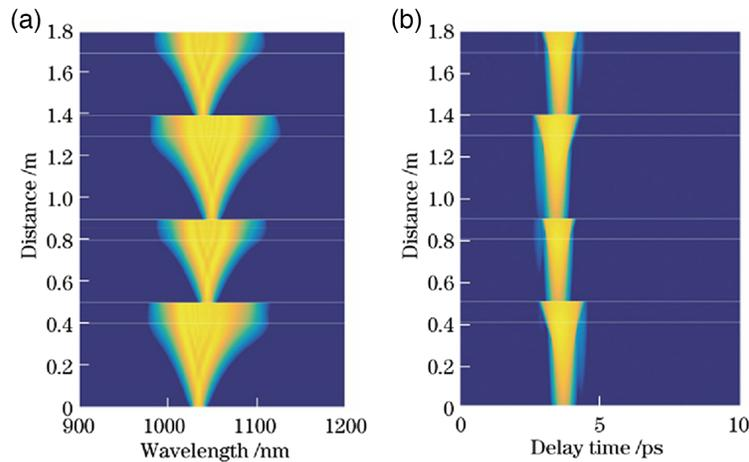
**Fig. 6** The pulse evolution diagram of multi-wavelength laser.<sup>35</sup> (a) The spectrum evolution of multi-wavelength laser; (b) the time domain evolution of multi-wavelength laser.
