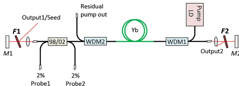
Fig. 3 Schematic diagram of the ultrashort pulse fiber generator.<sup>30</sup>
