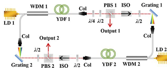
Fig. 12 Schematic of the Yb-doped Mamyshev oscillator based on NPE.<sup>73</sup>
