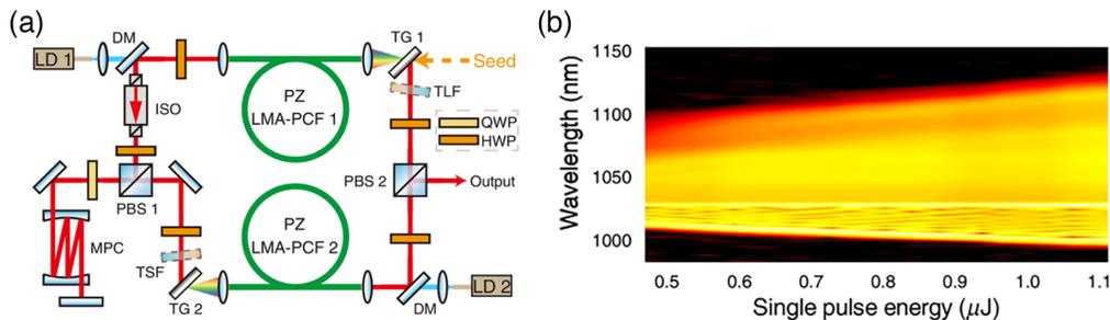
**Fig. 5** (a) Schematic of the polarizing LMA-PCF Mamyshev oscillator and (b) evolution of the output spectrum with the increase of pulse energy.<sup>34</sup>
