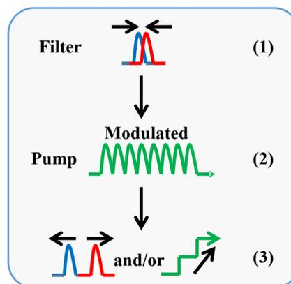
**Fig. 9** The starting process of self-starting Mamyshev oscillator with pump modulation and a moving filter.
