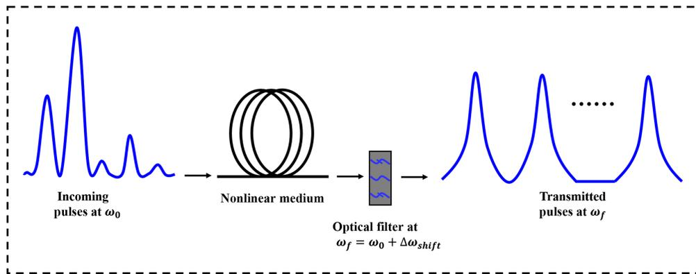
Fig. 1 Schematic of a single-pass MR.<sup>28</sup>
