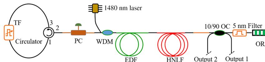
Fig. 13 Mode-locked Er-doped laser based on Mamyshev mechanism.<sup>75</sup>
