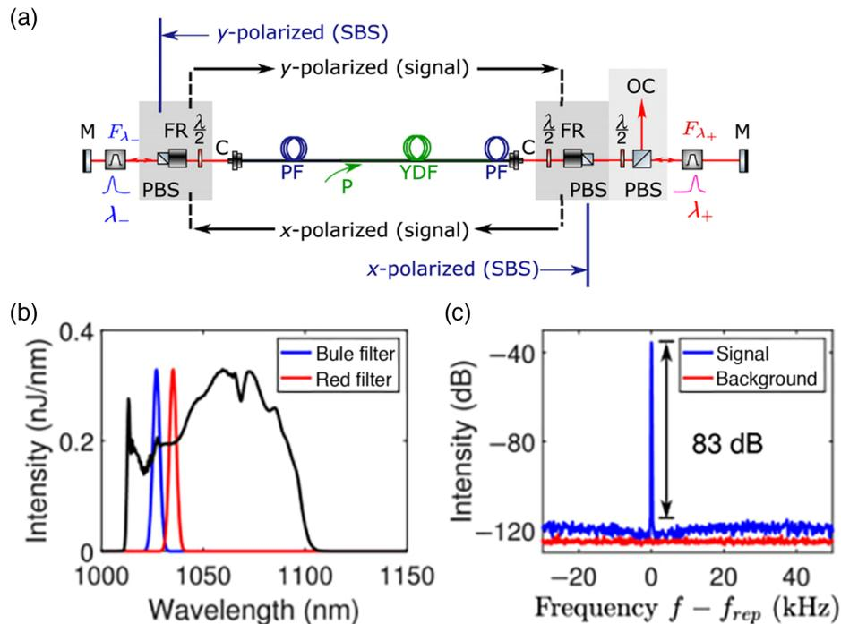
**Fig. 10** (a) Schematic of a damage-free linear Mamyshev oscillator with Faraday rotators; (b) spectra of delivered pulses and corresponding filters; and (c) RF spectrum  $f_{rep} = 16.1$  MHz.<sup>57</sup>
