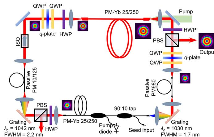
Fig. 7 The Mamyshev oscillator of femtosecond optical vortex beams.<sup>51</sup>
