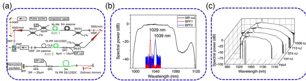
**Fig. 4** (a) experimental setup of the Mamyshev oscillator and the amplification arm; (b) output optical spectrum and the transmission spectra of the BPFs of Mamyshev oscillator; and (c) the optical spectrum of the input and the amplified signal of the amplification arm.<sup>33</sup>
