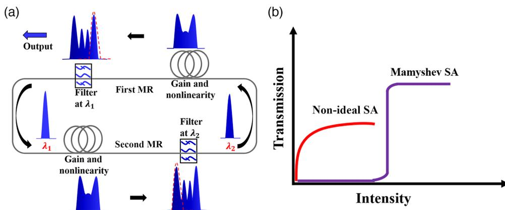
Fig. 2 (a) Schematic of a Mamyshev oscillator<sup>29</sup> and (b) comparison of Mamyshev SA and traditional non-ideal SA.
