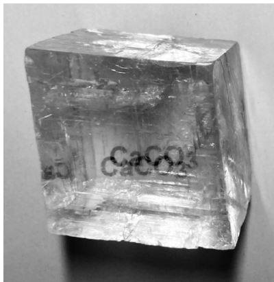
Figure 1.10 Birefringence of calcite splits the word beneath the crystal into two images. (Photograph by Sally Harris.)
