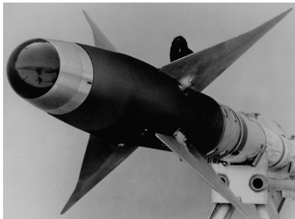
Figure 1.1 Nose of a Sidewinder missile showing the dome that protects the infrared seeker. (Photograph courtesy of Naval Air Warfare Center, China Lake, California.)
