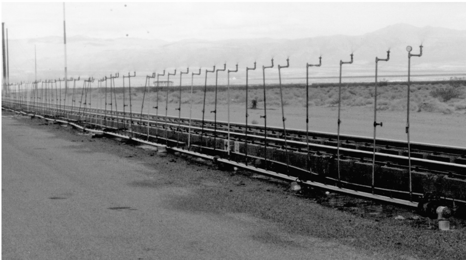
Figure 9.2 Upper: Dome mounted on a rocket sled at the Supersonic Naval Ordnance Research Track (SNORT) at the Naval Air Warfare Center at China Lake. 1 Lower: Spray heads used to create an artificial rainfield. (Photographs courtesy of Naval Air Warfare Center, China Lake.)
